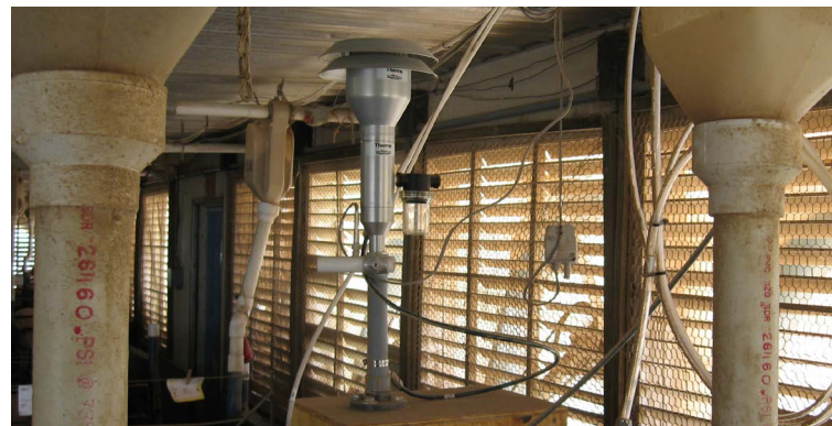
Researchers have positioned a sampling port and instruments in front of the primary exhaust fan in this building to measure exhaust gases, particulates, temperature, and relative humidity. Photo by Ken Casey.
